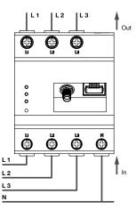
The device operates on phase L1
